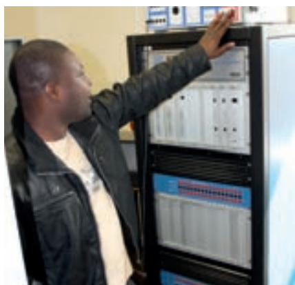
Doctor students A Adewole works on Hardware-in-the Loop simulation using the Real-Time Digital Simulator
